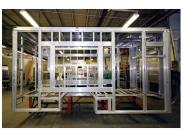
"DriveWorks configured the compartment sizes you see above, as well as the body length and height. These walls all have our custom proprietary extrusions that have been created as weldments in SOLIDWORKS."
